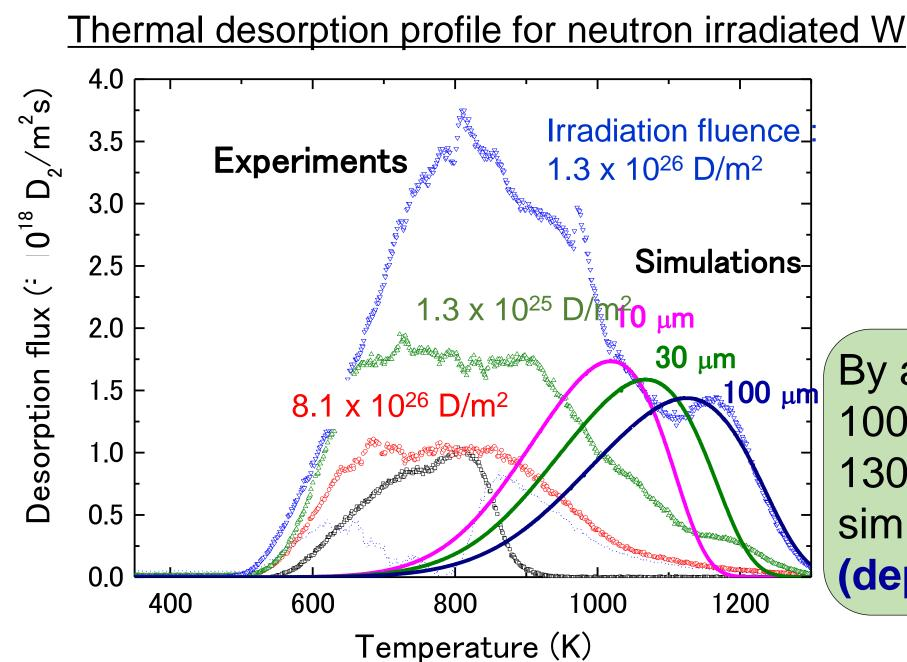
Neutron irradiation: 0.06 dpa, 563 K D plasma exposure at 473 K D retention:
