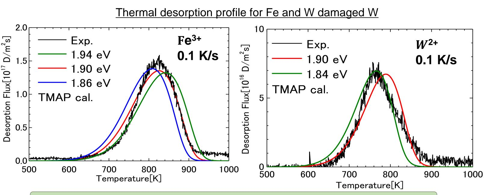
For both Fe and W damaged W, trap energies agree with 1.84-1.94 eV.
