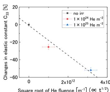
Fig.4 Changes in elastic constant due to helium implantation
