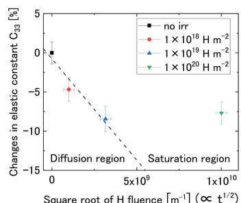
Fig.3 Changes in elastic constant due to hydrogen implantation
