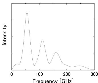
Fig. 2 The FFT spectrum, showing the acoustic-phonon resonances up to the 3rd overtones
